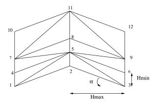
Figure 1: 2-D model boundary layer mesh
