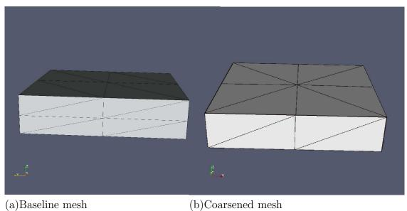
Figure 2: Semi-coarsening of a model boundary layer mesh. Note that the y-axis is scaled
