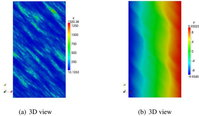
**Fig. 5** SPE10 permeability field and pressure solution
