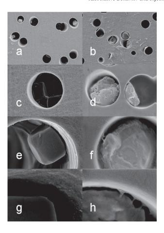
Figure 9 SEM images comparing a dry reference membrane previously exposed to standard brine (images a, c, e and g) and a dry membrane after the 2nd filtration of a solution of I20C12-0.5 at C=1 g/L and Q=500 mL/h (images b, d, f and h). Magnifications:  $\times 5\,000$  (a, b),  $\times 20\,000$  (c, d),  $\times 50\,000$  (e, f) and  $\times 100\,000$  (g, h). Average pore diameter is 2.6  $\mu$ m.
