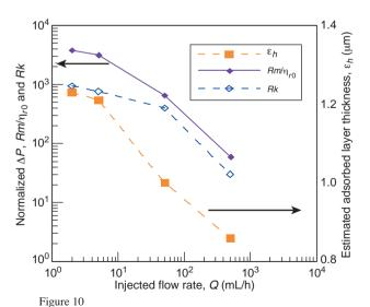
Normalized  $\Delta P$  plateau values,  $Rm/\eta_{n0}$  ( $\spadesuit$ ) and Rk ( $\diamondsuit$ ) (left axis), and polymer adsorbed layer thickness estimations,  $\varepsilon_h$  ( $\blacksquare$ ) (right axis), determined during the 2nd filtrations of 1 g/L solutions of I20C12-0.5 at flow rates ranging from 2 to 500 mL/h, corresponding to initial wall shear rates  $\dot{\gamma}_{wall}$  ranging from 15 to 3 800 s<sup>-1</sup>.
