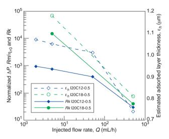
Figure 14 Impact of the chemical composition for different flow rates: extrapolated plateau values of Rk (filled symbols) and  $\varepsilon_h$  (open symbols) values determined during 2nd filtrations of I20C12-0.5 ( $\blacklozenge$  and  $\diamondsuit$ ) and I20C18-0.5 ( $\blacklozenge$  and  $\diamondsuit$ ) at 1 g/L and flow rates ranging from Q=2 mL/h to Q=500 mL/h. Lines are guides for the eyes.
