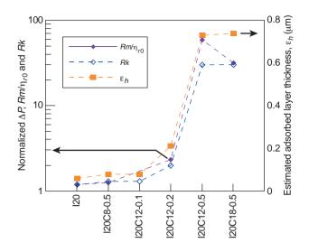
Figure 13 Impact of the chemical composition: normalized  $\Delta P$  plateau values,  $Rm/\eta_{r0}$  ( $\blacklozenge$ ) and Rk ( $\diamondsuit$ ) (left axis) and polymer adsorbed layer thickness estimations,  $\varepsilon_h$  ( $\blacksquare$ ) (right axis), determined for the 2nd filtrations of the full set of polymers injected at C=1 g/L and Q=500 mL/h. Discontinuous junctions between dots are guides for the eyes.
