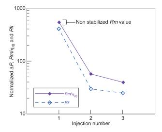
Normalized pressure drops,  $Rm/\eta_{r0}$  ( $\spadesuit$ ) and Rk ( $\diamondsuit$ ), determined for the 3 successive filtrations of the same solution of I20C12-0.5 in 3 different membranes. Values for the 1st filtration were determined at the maximum volume injected (about 2 500 mL), values for the 2nd and 3rd filtrations correspond to extrapolated plateau values; C=1 g/L, Q=500 mL/h.
