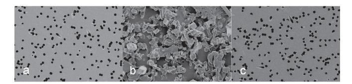
SEM images of a reference membrane dried a) after having been exposed to standard brine, b) of dried membranes after the 1st c) and the 2nd filtration of the same solution of I20C12-0.5 at C = 1 g/L and Q = 500 mL/h. Magnification × 1000. Average pore diameter is 2.6  $\mu$ m.
