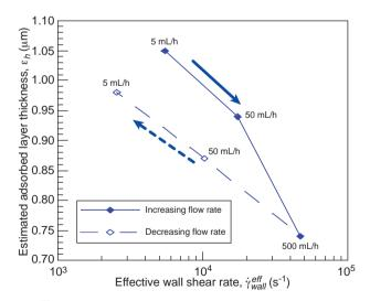
Figure 11 Estimated adsorbed layer thickness  $(\varepsilon_h)$  *versus* the effective wall shear rates  $(\dot{\gamma}_{wall}^{eff})$  determined by exposing the adsorbed layer (formed during the injection of I20C12-0.5 at 5 mL/h) to brine flow rates ranging from 5 to 500 mL/h  $(\spadesuit)$  and then to flow rates ranging from 500 to 5 mL/h  $(\diamondsuit)$ .
