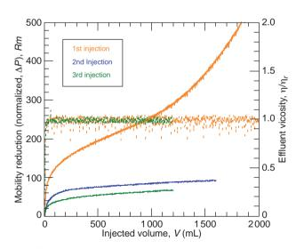
Successive frontal filtration of the same I20C12-0.5 solution in three different membranes – Rm curves (lines) and  $\eta/\eta_P$  (dots) from on-line capillary tube measurements; C = 1 g/L, Q = 500 mL/h. The stabilization trend observed from the 2nd filtration is typical of all HMWSP and WSP investigated in this study.
