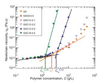
Figure 5 Newtonian viscosity ( $\eta_0$ ) vs polymer concentration (C) for the 5 HMWSP investigated and the reference WSP. The straight lines allow estimating  $C^*$  and  $C\eta$  (see text for definition).
