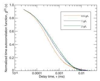
Figure 3 Normalized DLS time autocorrelation functions  $(g^{(2)}(\tau))$  obtained with I20C12-0.5 at 0.5 g/L, 1 g/L and 2 g/L in standard brine
