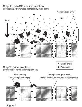
Schematic of the three main mechanisms potentially involved in HMWSP-induced permeability impairment (accumulation layer, pore blocking and adsorption on pore walls) of the membrane during the filtration of HMWSP, according to experimental procedure implemented.
