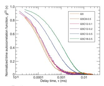
Figure 4 Normalized DLS time autocorrelation functions  $(g^{(2)}(\tau))$  showing the impact of the chemical composition of the HMWSP compared to WSP. All measurements were carried out at 1 g/L polymer concentration.
