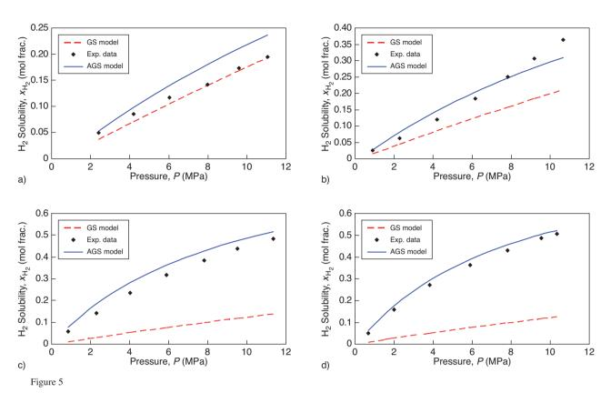
Solubility of hydrogen on heavy petroleum cuts. a) in LVGO at 603 K, b) in HVGO a 653 K, c) in ABVB at 523 K, d) in GDAR at 523 K.
