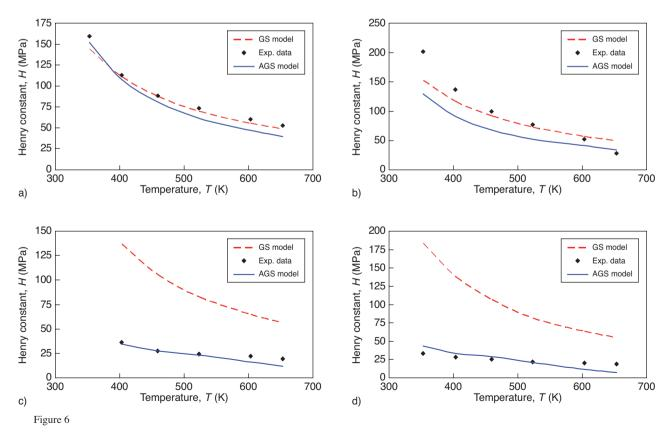
Henry constant of hydrogen in heavy petroleum cuts. a) in LVGO, b) in HVGO, c) in ABVB, d) in GDAR.
