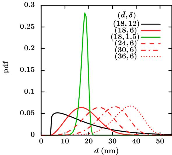
FIG. 2: (Color online) Weibull distribution functions used in this study to generate networks, labelled according to their mean diameter and standard deviation  $(\bar{d}, \delta)$ . Solid lines correspond to the same mean diameter  $\bar{d} = 18$  nm, while dashed and dotted lines correspond to the same standard deviation  $\delta = 6$  nm. The minimum diameter (see Eq. 16) is  $d_{min} = 4$  nm.
