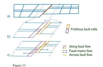
Fault as a zone; a) sketch of a fault grid; b) zoom on the fault zone and corresponding fictitious cells as introduced in the double interface fault model; c) illustration of the different fluxes that appear in mass balance equation for the fictitious fault cells.
