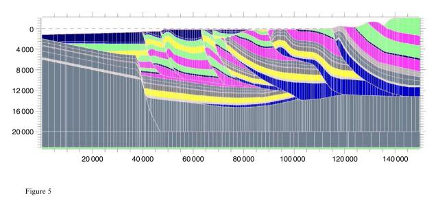
Example of a 2D multi-block grid used in Ceres (Vilasi et al., 2009). The vertical lines are the vertical pillars of the different blocks.
