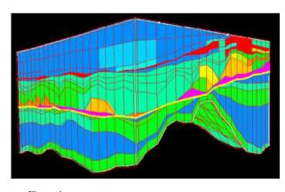
Figure 4 Example of a 3D vertical pillar grid (Schneider *et al.*, 2000).
