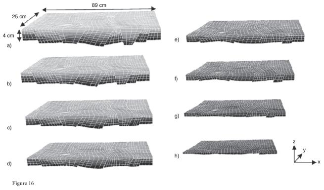
8 incremental volumetric restoration steps. Color represents the layer number or the stratigraphic event. a) Initial structural model; b) to h) successive snapshots during the model evolution. Hexahedra mesh nearly everywhere for a better coupling with the fluid flow simulator. The topmost horizon is restored to a flat datum. Sliding along the faults is done without any gap or overlap.
