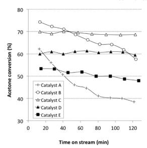
Fig. 2 Acetone conversion as a function of time on stream. Operating conditions:  $T = 200 \, ^{\circ}\text{C}$ ,  $P = 3 \, \text{bar}$ , WHSV =  $1 \, \text{h}^{-1}$  (1 g of catalyst, acetone = 1 g  $h^{-1}$ ),  $N_2 = 9 L h^{-1}$ ,  $H_2 = 1 L h^{-1}$ . Conversion based on carbon weight.
