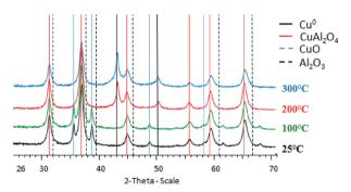
Fig. 1 XRD patterns of catalyst C after reduction for 30 min at different temperatures. Phases: CuO (ICDD PDF No. 04-005-4712); CuAl<sub>2</sub>O<sub>4</sub> (ICDD PDF No. 04-015-0578); Cu<sup>0</sup> (ICDD PDF No. 04-003-1450); Al<sub>2</sub>O<sub>3</sub> (ICDD PDF No. 10-0425).
