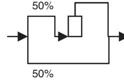
Phase 2: 100% flue gas treated at 90% capture rate
