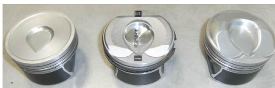
Figure 1: Piston geometries to obtain the three different CRs (left: CR=7.5:1, middle: CR=10.5:1 (stock), right: CR=12:1)
