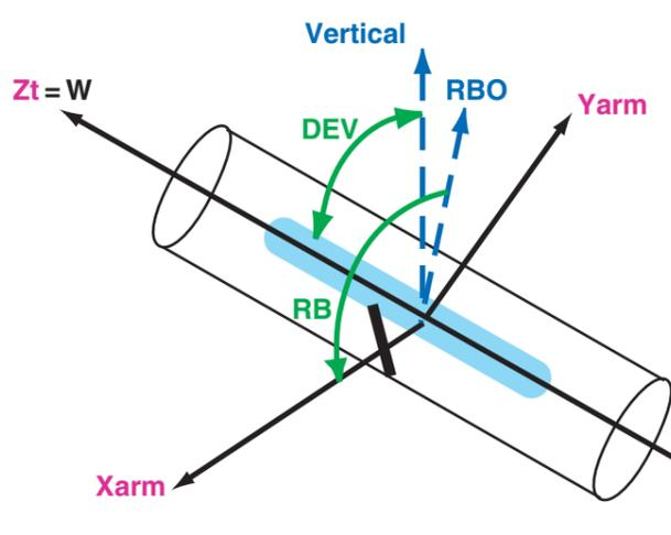
Recorded orthogonal components are fixed in the tool :
