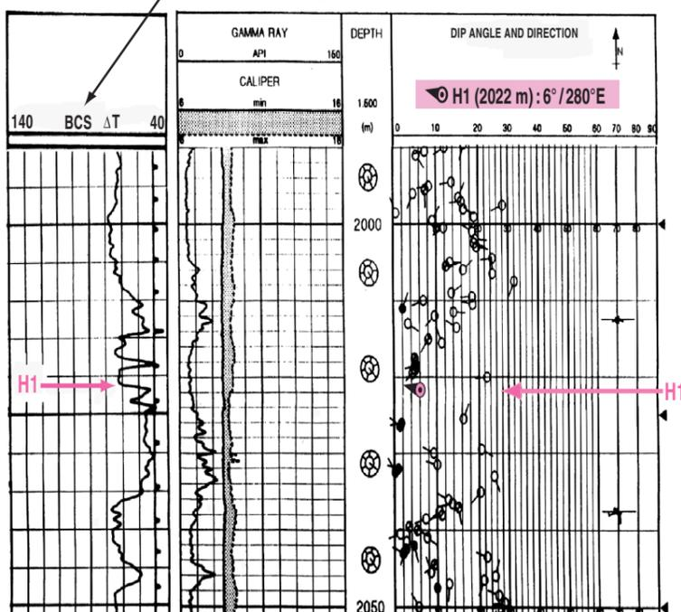
6 arm Dipmeter results on Tad pole plot
