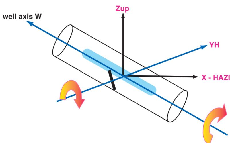
In the **BINNACLE** setting, one gimbal is free to rotate around the (Xarm) axis orthogonal to the tool axis (W) in the plane of arm opening, but with an unknown orientation; the other gimbal is free to rotate around the horizontal axis (YT).
