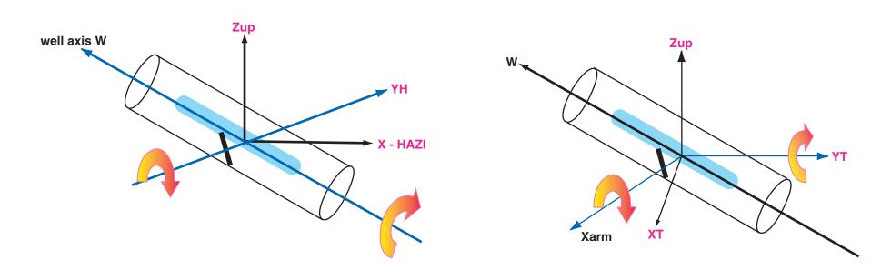
in near vertical well (DEV < 8°), an orientation accessory such as a gyroscope or a inclinometer / magnetometer has to be combined with the VSP tool, without deteriorating the mechanical VSP tool coupling to the formation or generating unwanted power induced seismic noise on the tool geophones. Commercial inclinometer / magnetometers are widely used in wireline logging, and</li>
