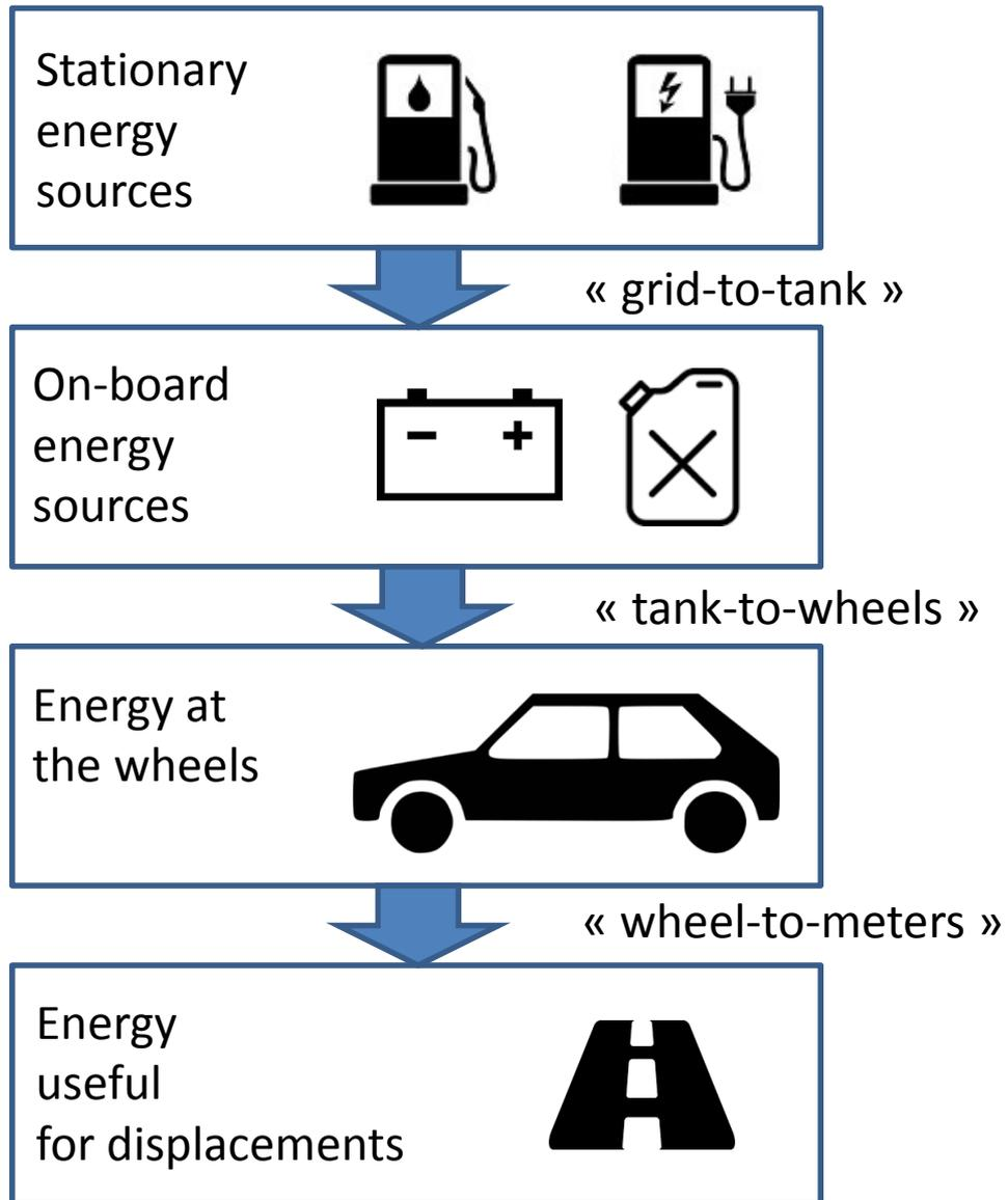
Figure 1: The three main energy conversion steps for road vehicles.
