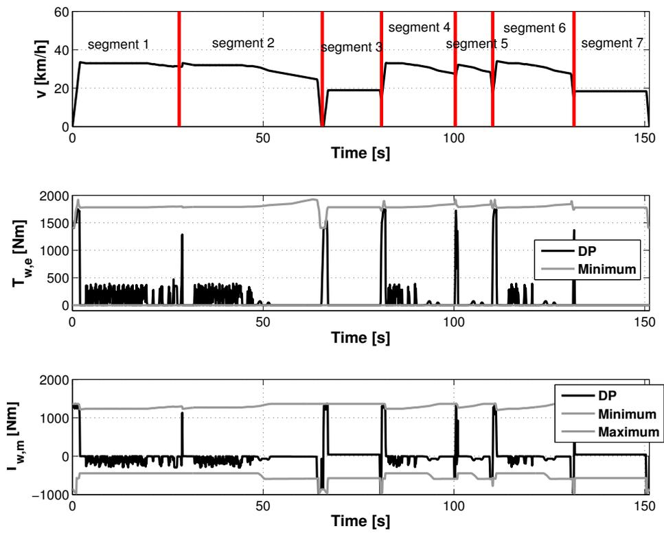
Figure 10: DP trajectories for an HEV, seven consecutive segments. From top to bottom, the figures show speed  $v$ , torque at the wheels from the engine,  $T_{w,e} := T_e \gamma_e$ , and torque at the wheels from the motor  $T_{w,m} := T_m \gamma_m$  as a function of time.
