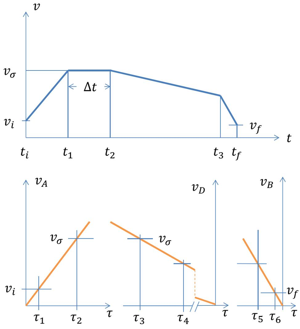
Figure S6: Graphical illustration of the parametric optimization method in the case of a four-phase optimal trajectory. Upper plot shows the speed trajectory with the switching times  $t_1, \dots, t_3$  and the singular arc  $v_\sigma$ . Lower plots show the trajectories  $v_A(\tau)$ ,  $v_D(\tau)$ , and  $v_B(\tau)$  together with the characteristic times  $\tau_1, \dots, \tau_6$ .
