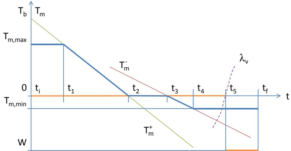
Figure 4: Qualitative control trajectories for an EV, for the mode sequence SA-A-C-D-SD-B. Shown in the picture are motor and brake torques  $T_m^*$  (blue),  $T_b^*$  (orange), auxiliary functions  $T_m^+$  (green) and  $T_m^-$  (brown) defined in the main text, and velocity costate  $\lambda_v$  (dashed purple) as a function of time. Switching times are such that  $T_m^+(t_1) = T_{m,max}$ ,  $T_m^+(t_2) = 0$ ,  $T_m^-(t_3) = 0$ ,  $T_m^-(t_4) = T_{m,min}$ ,  $\lambda_v(t_5) = 0$ .
