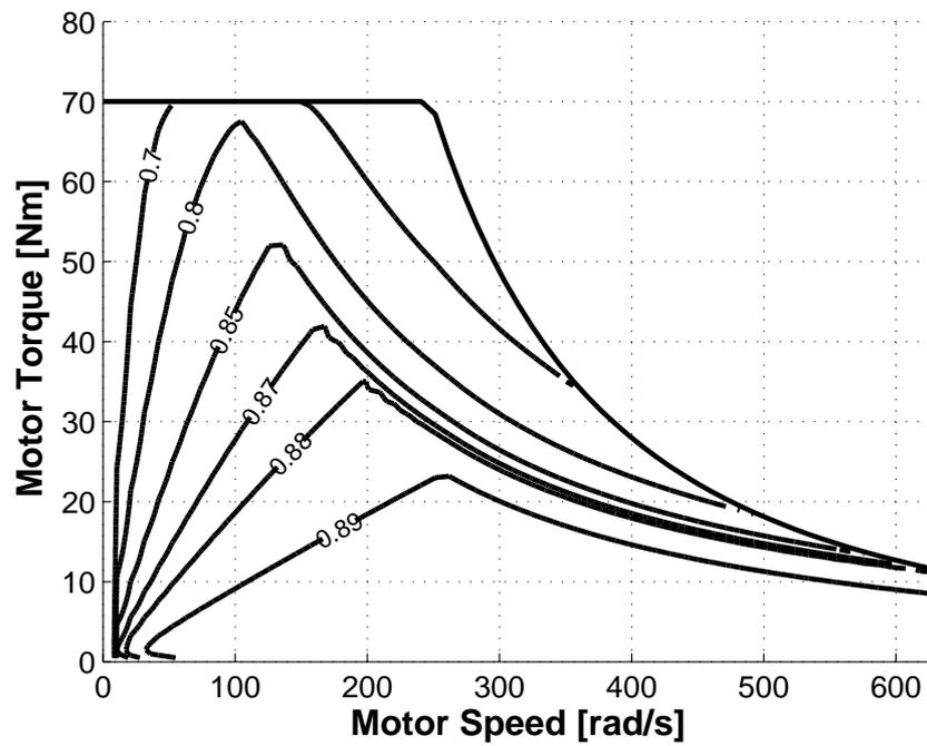
Figure S3: Typical efficiency map of an EV electric motor. The figure shows equal efficiency contours (labelled), as well as maximal torque curve  $T_{m,max}$ . When specific data are not available, second quadrant, that is, negative torque values (generating mode) may be estimated by mirroring the first quadrant.
