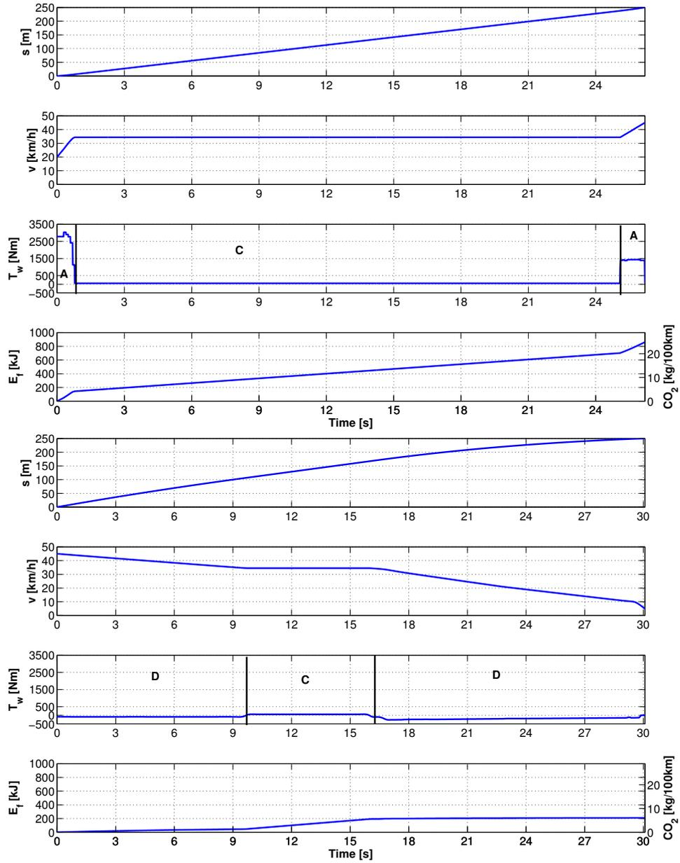
Figure 8: DP trajectories for an ICEV,  $v_i = 20$  km/h,  $v_f = 45$  km/h,  $t_f \approx 26$  s (top),  $v_i = 45$  km/h,  $v_f = 5$  km/h,  $t_f = 30$  s (bottom),  $s_f = 250$  m,  $\alpha = 0$ . From top to bottom, the figures show position  $s$ , speed  $v$ , torque at the wheels  $T_w := r_w F_w$ , and fuel energy consumption  $E_f$  as a function of time. Labels to the wheel torque refer to the control modes introduced in the main text.
