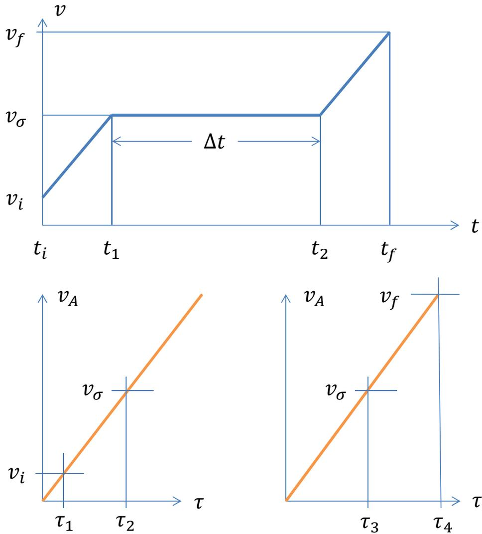
Figure S5: Graphical illustration of the parametric optimization method in the case of a three-phase optimal trajectory. Upper plot shows the speed trajectory with the switching times  $t_1, t_2$  and the singular arc  $v_\sigma$ . Lower plots show the trajectory  $v_A(\tau)$  together with the characteristic times  $\tau_1, \dots, \tau_4$ .
