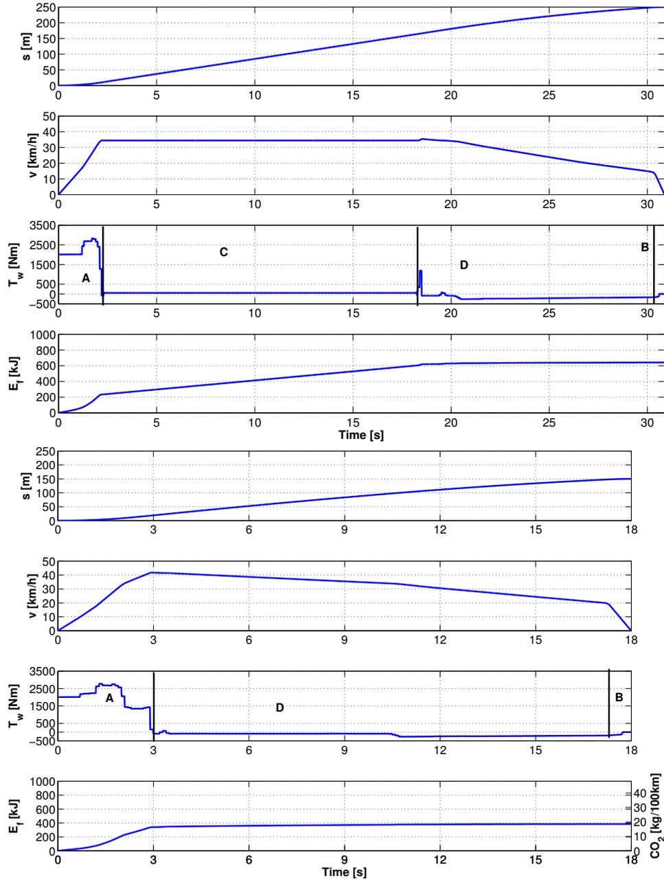
Figure 7: DP trajectories for an ICEV,  $s_f = 250$  m,  $t_f \approx 30$  s (top),  $s_f = 150$  m,  $t_f = 18$  s (bottom),  $v_i = v_f = \alpha = 0$ . From top to bottom, the figures show position  $s$ , speed  $v$ , torque at the wheels  $T_w := r_w F_w$ , and fuel energy consumption  $E_f$  as a function of time. Labels to the wheel torque refer to the control modes introduced in the main text.
