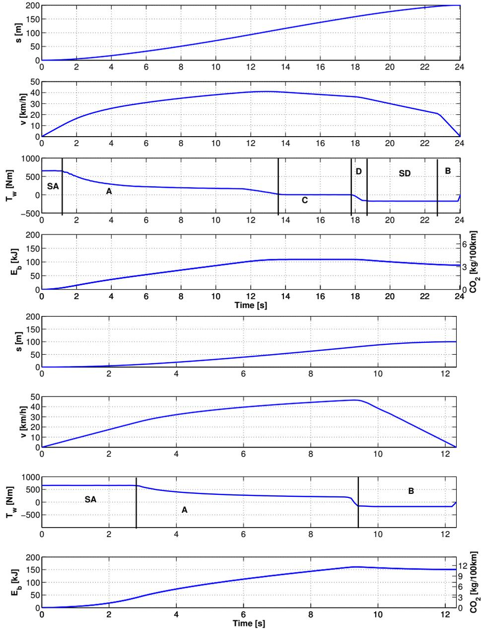
Figure 6: DP trajectories for an EV,  $s_f = 200$  m,  $t_f = 24$  s (top),  $s_f = 100$  m,  $t_f \approx 12$  s (bottom),  $v_i = v_f = \alpha = 0$ . From top to bottom, the figures show position  $s$ , speed  $v$ , torque at the wheels  $T_w := r_w F_w$ , and battery energy consumption  $E_b$  as a function of time. Labels to the wheel torque refer to the control modes introduced in the main text.
