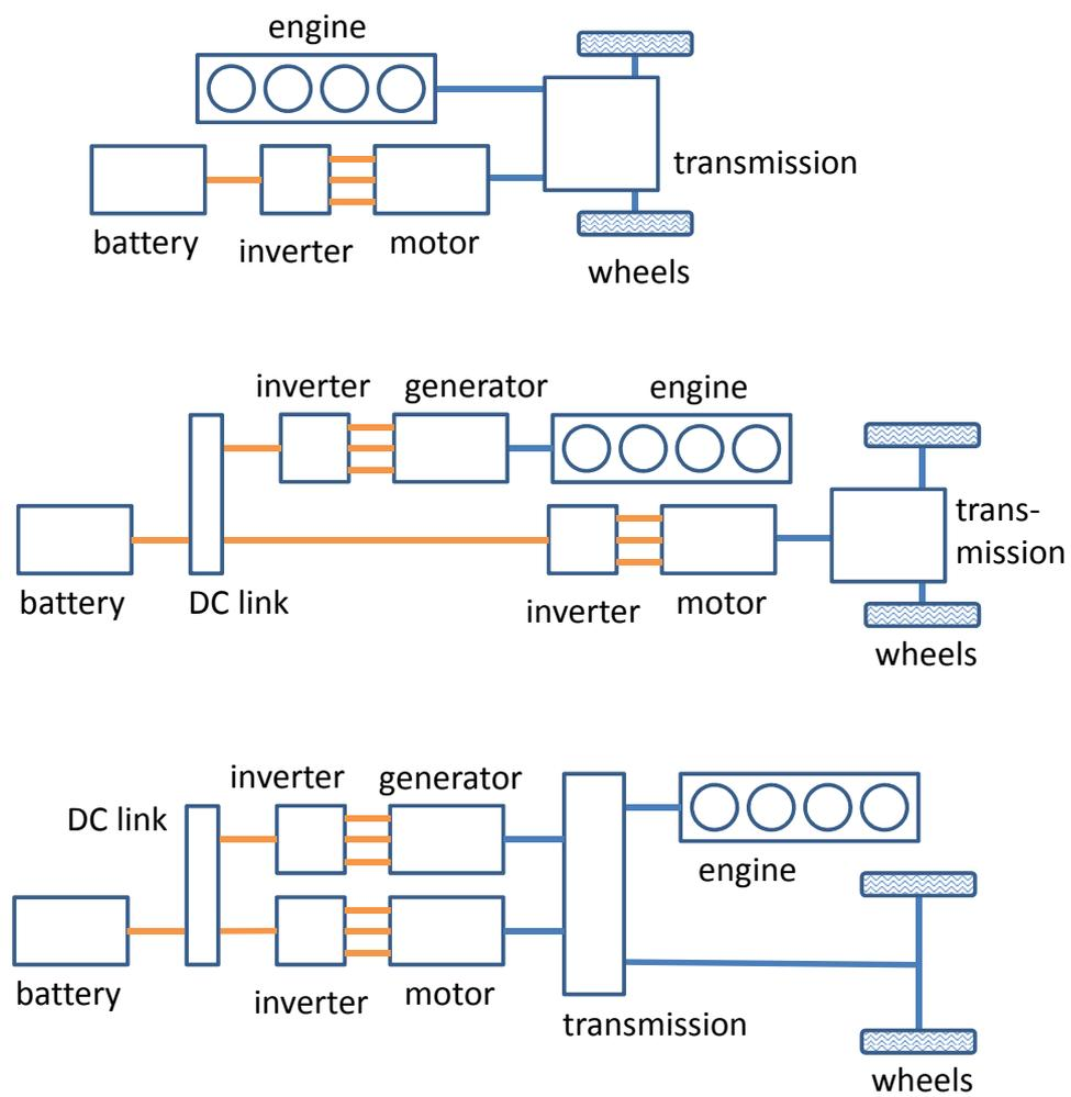
Figure S4: General layout of a parallel HEV (top), a series HEV (middle), and a series-parallel HEV (bottom). Blue bold lines between subsystems represent mechanical power, orange bold lines represent electrical power.
