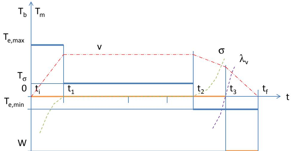
Figure 5: Qualitative control and speed trajectories for an ICEV, for the mode sequence A-C-D-B. Shown in the picture are engine and brake torques,  $T_e$  (blue),  $T_b$  (orange), vehicle speed  $v$  (dashdot red), auxiliary function  $\sigma$  (dashed green) defined in the main text, and velocity costate  $\lambda_v$  (dashed purple) as a function of time. Switching times are such that  $\sigma(t_1) = 0$ ,  $\sigma(t_2) = 0$ ,  $\lambda_v(t_3) = 0$ .
