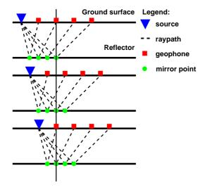
Fig. 7. Seismic acquisition for one horizontal layer and three different shot points.
