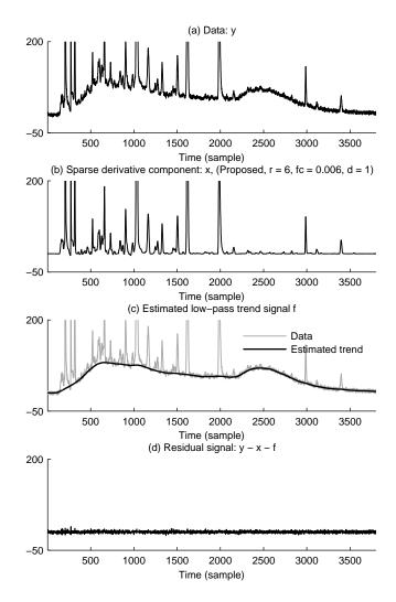
Figure 13: Processing of noisy chromatogram data using BEADS. (a) Chromatogram data with additive noise. (b) Estimated peaks. (c) Estimated baseline. (d) Residual.
