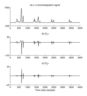
Figure 1: Gas chromatogram from two-dimensional gas chromatography [52], with flat baseline and low noise: (a) analytical signal  $\mathbf{x}$ , (b) first-order difference  $\mathbf{D}_1\mathbf{x}$  and (c) second-order difference  $\mathbf{D}_2\mathbf{x}$ . The chromatographic signal is sparse, as are its first- and second-order derivatives.
