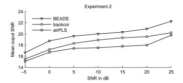
Figure 8: Experiment 2. Output SNR as a function of input SNR.
