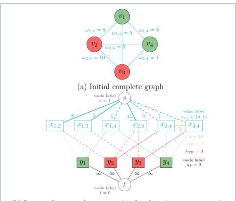
(b) Intermediate graph construction for the min-cut computation
