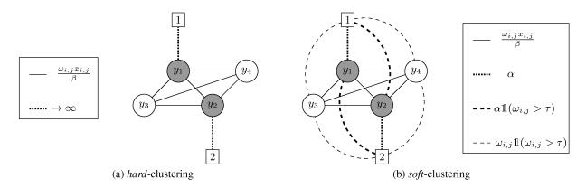
Figure 2. Graph built to perform (a) hard- and (b) soft-clustering. We define as many markers as  $\mathrm{TFs}$  (gray nodes), labeled with  $\mathrm{TF}$  indices. In the hard-clustering case, optimization constrains all node labels y to be equal to one of the markers. For soft-clustering, thanks to weights  $\mu_{i,j}$ , two clusters are merged if their respective  $\mathrm{TFs}$  have strong weights. Legend-box  $\alpha$  parameter for soft-clustering refers to (7).
