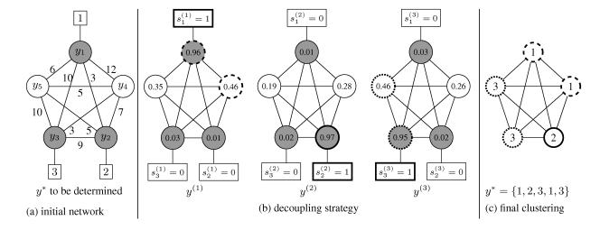
Figure 3. Graph-based clustering using a decoupling strategy for *hard*-clustering. The principle is similar for *soft*-clustering. Gray nodes represent TFs nodes. The T-label problem is decomposed into T binary sub-problems by setting the component t of marker labels  $s^{(t)}, t \in \mathbb{T}$ , to one and the others to zero. Each sub-problem t leads to a probability for each node. The final node clustering corresponds to the label whose probability amidst the T sub-problems is maximal.
