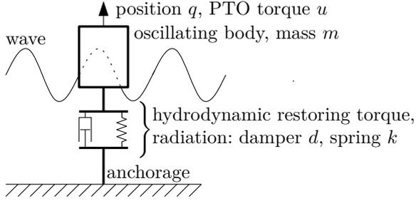
Fig. 1. Simplified model of a wave energy generator.
