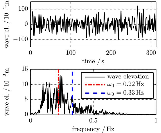
Fig. 2. Wave recorded at Galway Bay in the time and frequency domain.
