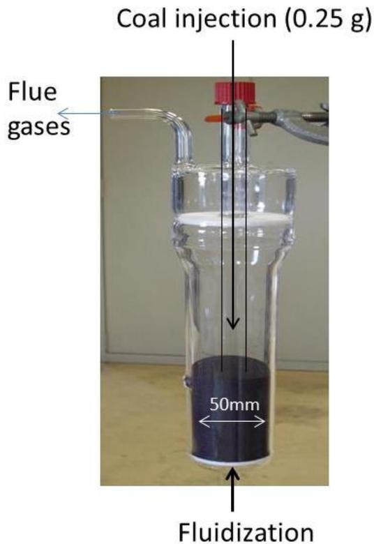
Figure 5: 50 mm i.d. batch fluidized bed reactor for solid fuel Chemical Looping Combustion [35]
