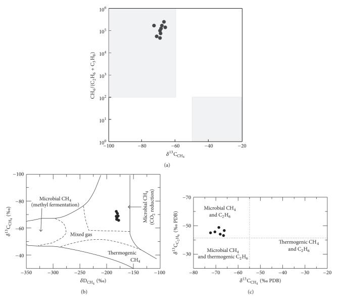
FIGURE 4: Diagrams for the study venting gases of the Aquitaine Shelf of (a)  $\delta^{13}C_{CH_4}$  versus methane to (ethane and propane) molecular composition ratio (modified after Bernard et al., 1978); (b)  $\delta^{13}D_{CH_4}$  versus  $\delta^{13}C_{CH_4}$  (modified after Schoell, 1983, and Whiticar, 1999); and (c)  $\delta^{13}C_{CH_4}$  versus  $\delta^{13}C_{CH_4}$  (modified after Bernard et al., 1978).
