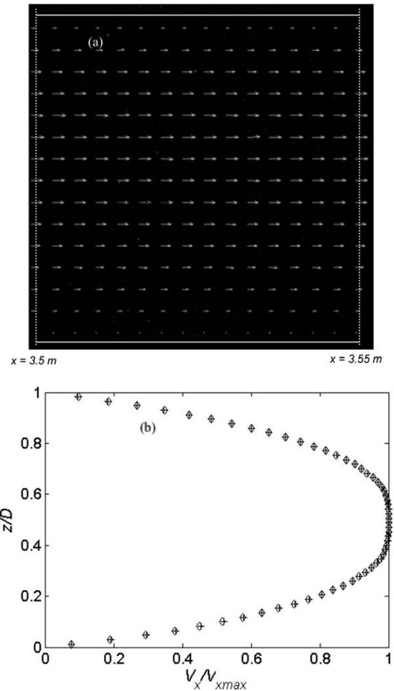
**Figure 5. (a) Instant velocity field for  $U_m = 0.85 \text{ m s}^{-1}$ ; (b) axial velocity profiles at  $x = 3.5 \text{ m}$  ( $\pi$ ) and  $x = 3.55 \text{ m}$  ( $+$ ).**
