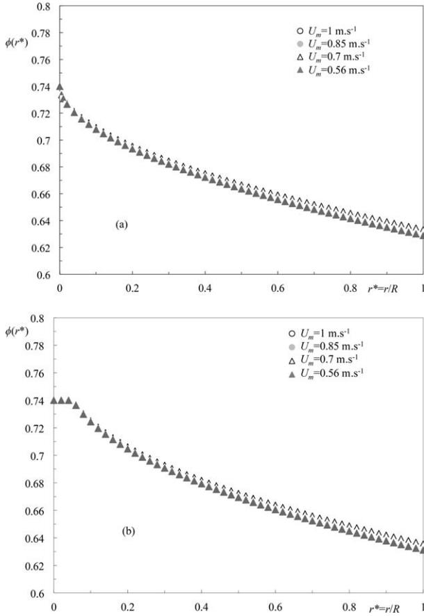
**Figure 12. Dispersed phase concentration radial profiles from Eq. 13.**
