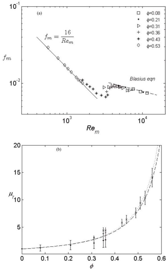
**Figure 1. (a) Wall friction factor as a function of the mixture Reynolds number at various concentrations ( $Re_m = \rho_m U_m D / \mu_m$ ) from Pouplin et al.<sup>6</sup>; (b) relative viscosity as a function of oil volume fraction ( $\phi_M = 0.74$ ).**
