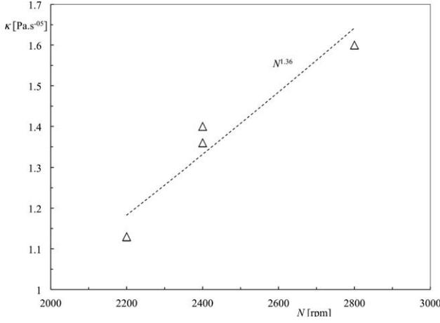
**Figure 11. Consistency factor  $\kappa$  vs. pump rotation speed  $N$ .**
