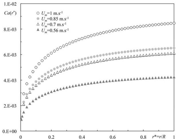
**Figure 15. Capillary number as function of radial position in the pipe cross section.**
