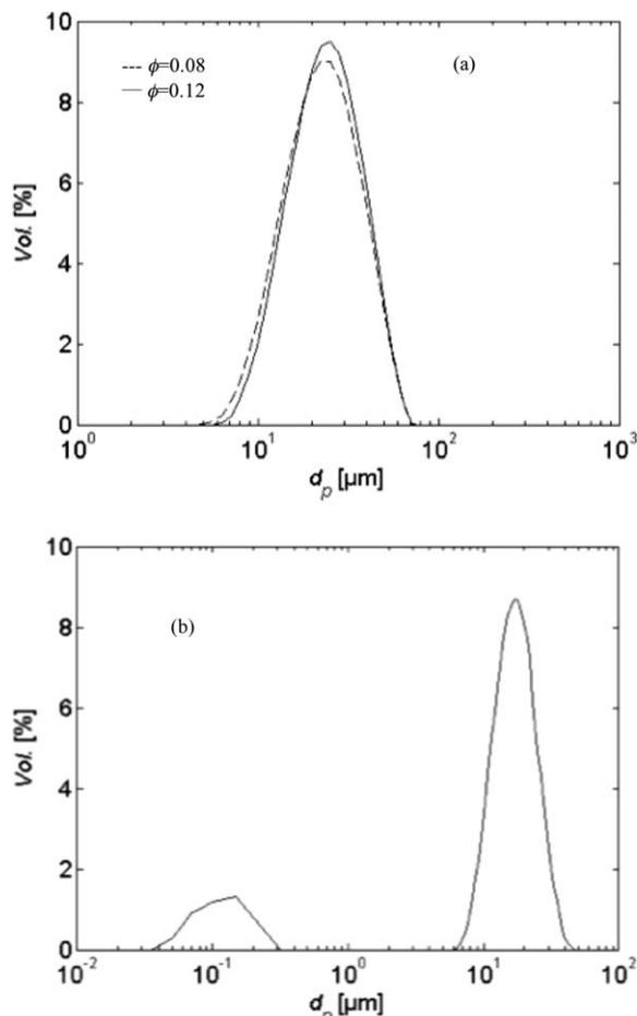
**Figure 3.** Drop size distribution at low concentration (a)  $N = 1900$  rpm; (b)  $N = 2400$  rpm. Continuous line (oil volume fraction of 12%); dashed line (oil volume fraction of 8%).
