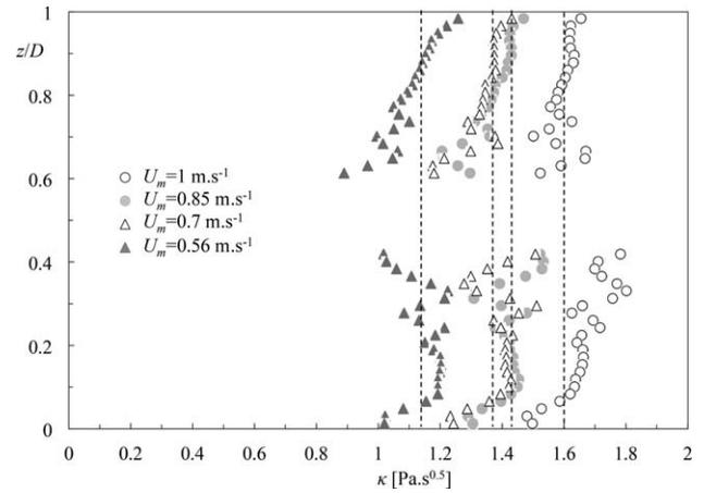
**Figure 9. Profiles of consistency factor  $\kappa$  in the cross-section at different mixture velocities.**
