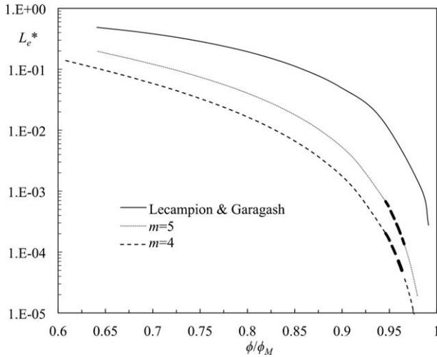
**Figure 17. Evolution of length of establishment as a function of concentration derived from model of Lecampion and Garagash.<sup>24</sup>**
