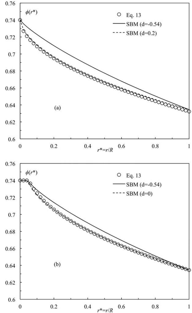
**Figure 13. Comparison of SBM predictions (Eq. 14) with theoretical profile of  $\phi$  as derived from Eq. 13.**
