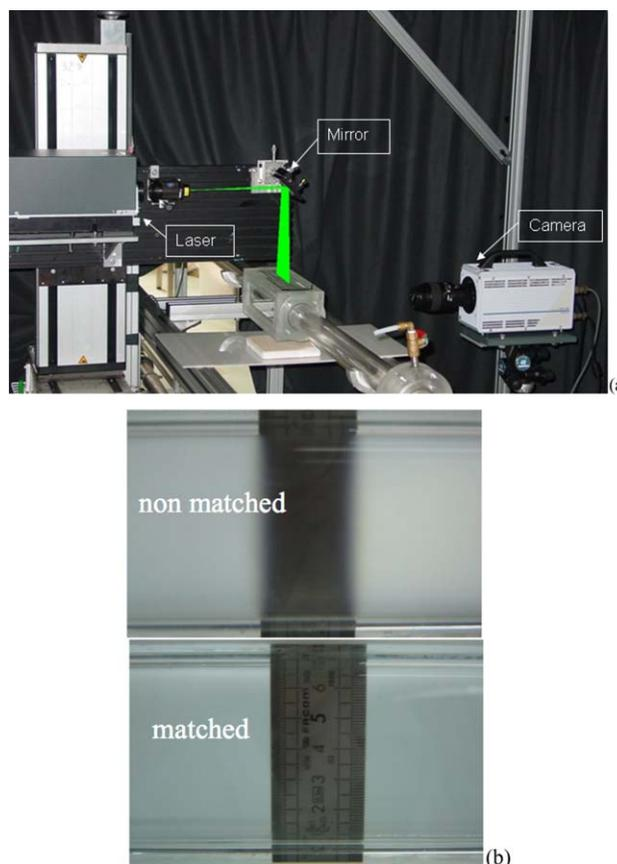
**Figure 4.** (a) PIV system implemented on the pipe; (b) illustration of phase index matching in the pipe flow.
