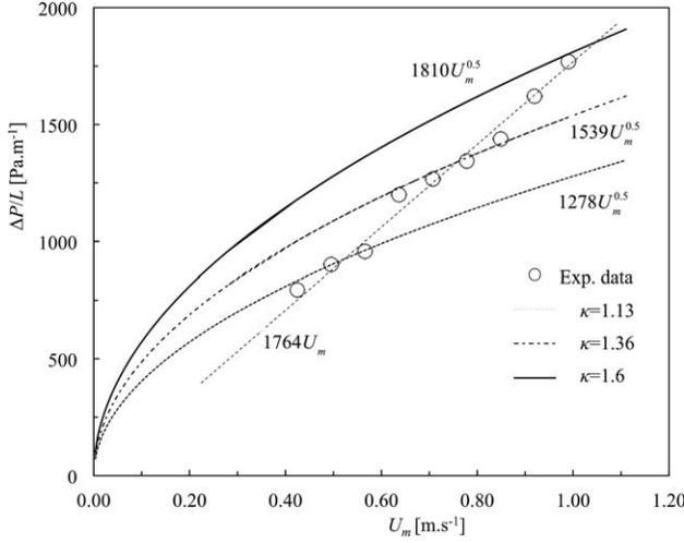
Figure 10. Pressure drop vs. mixture velocity.
