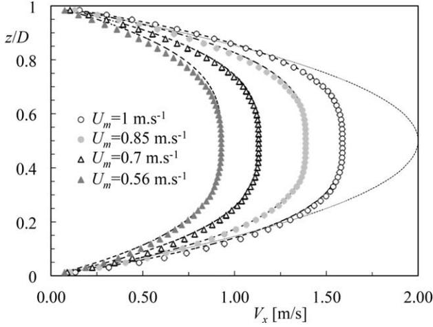
**Figure 6. Axial velocity profiles in the cross section at different mixture velocities.**
