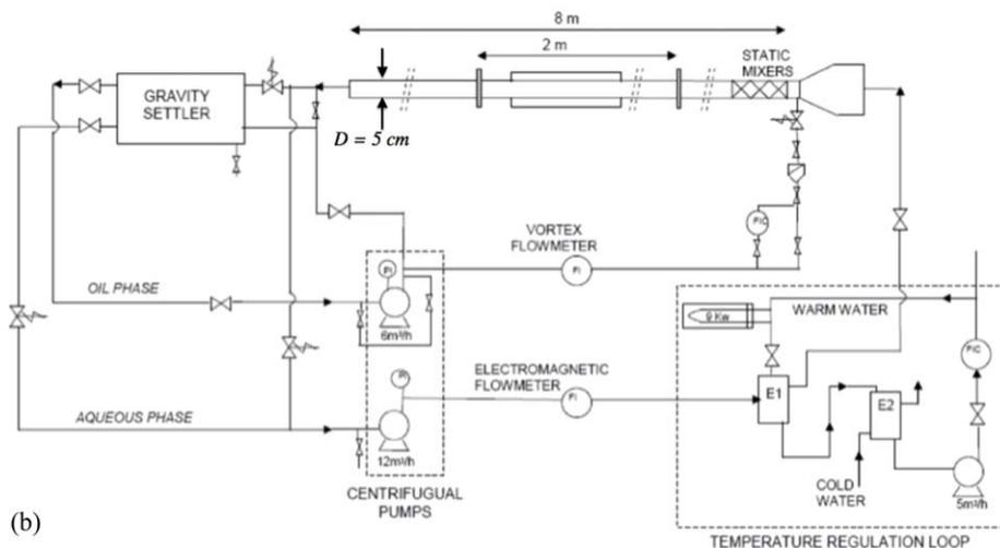
**Figure 2. Overview (a) and schematic (b) of the experimental rig.**
