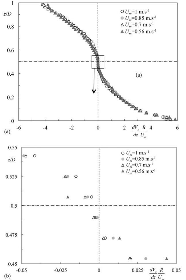
**Figure 7. (a) Velocity gradient profiles in the cross-section at different mixture velocities (b) Zoom near the centerline.  $R$  is the pipe radius ( $=2.5\text{cm}$ ).**
