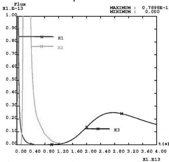
Fig. 6.1: Output mass flux for the three flow regimes
