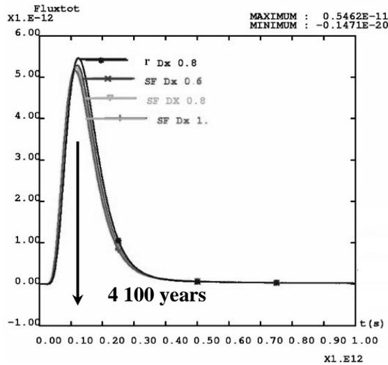
Fig. 8: total flux at the outlets for the more diffusive regime (K3)
