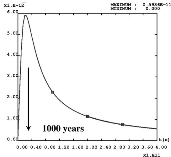
Fig. 10.3: Total mass flow (with matrix diffusion)
