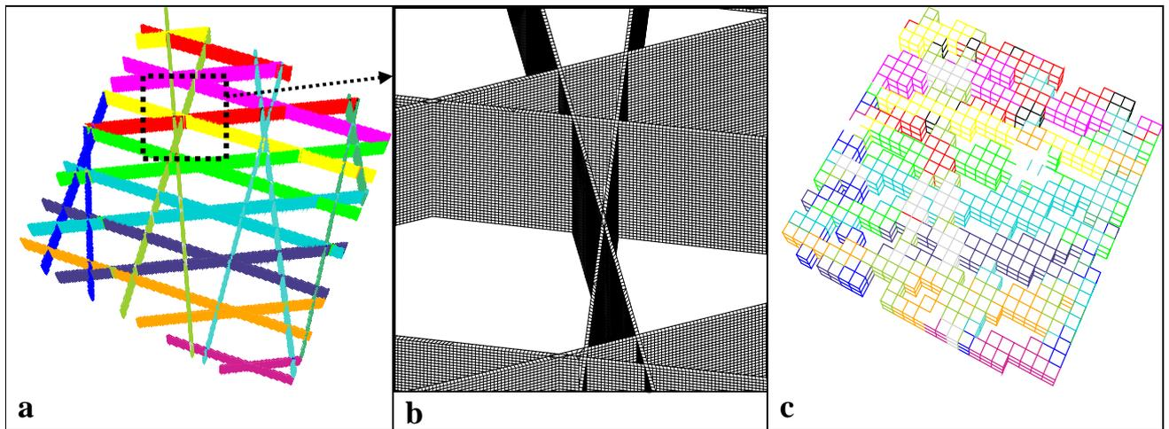
508 Fig. 6. Discretization of a regular fracture network by using a fine grid size of 0.2 m on a side (a)
