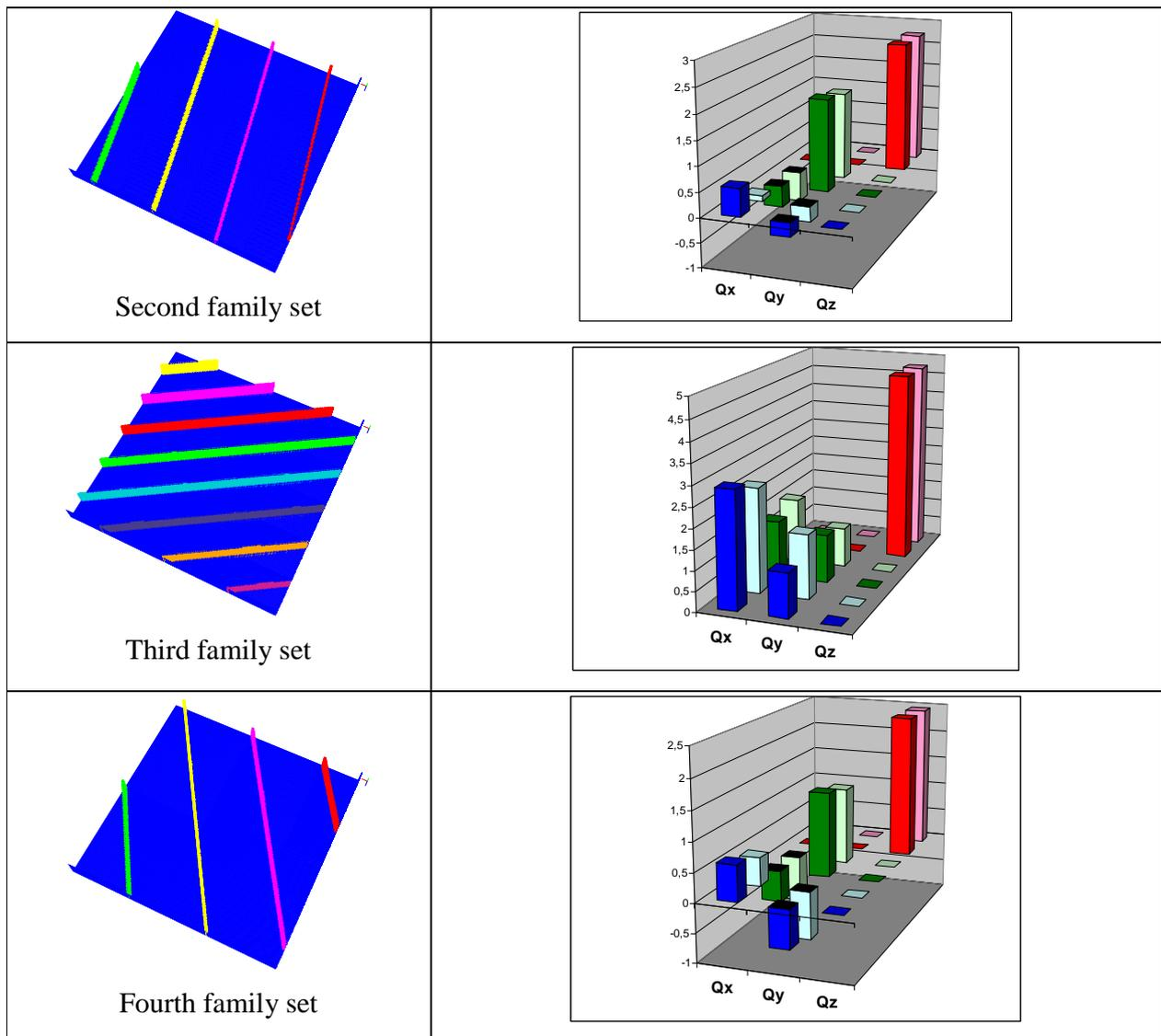
511 Fig. 7. Calculations of fluxes in a block enclosing different families of parallel fractures.  $Q_x$ ,  $Q_y$ ,
