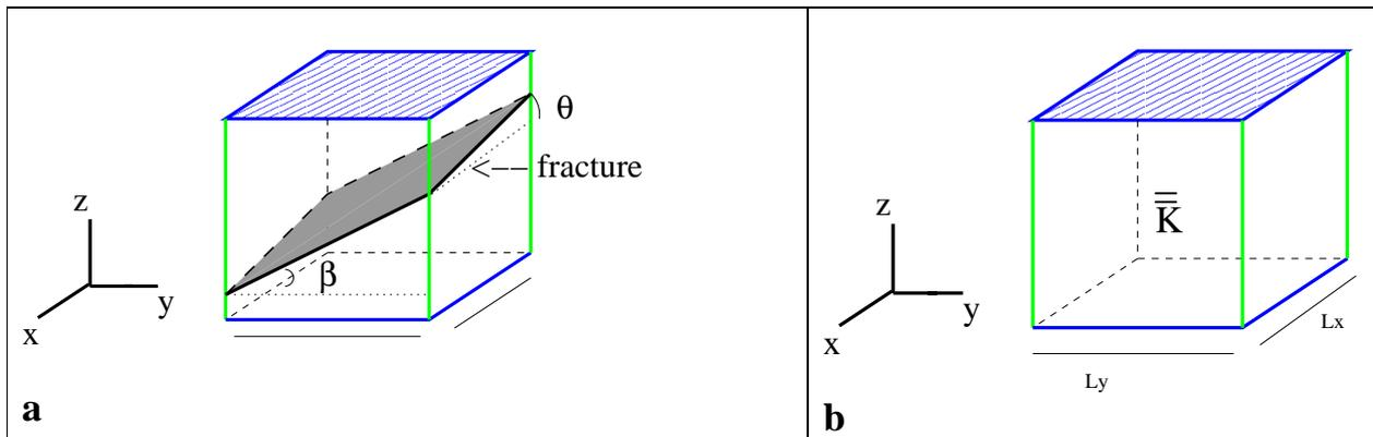
249 Fig. 4. A cell enclosing a portion of fracture (4a) and the equivalent hydraulic conductivity tensor
