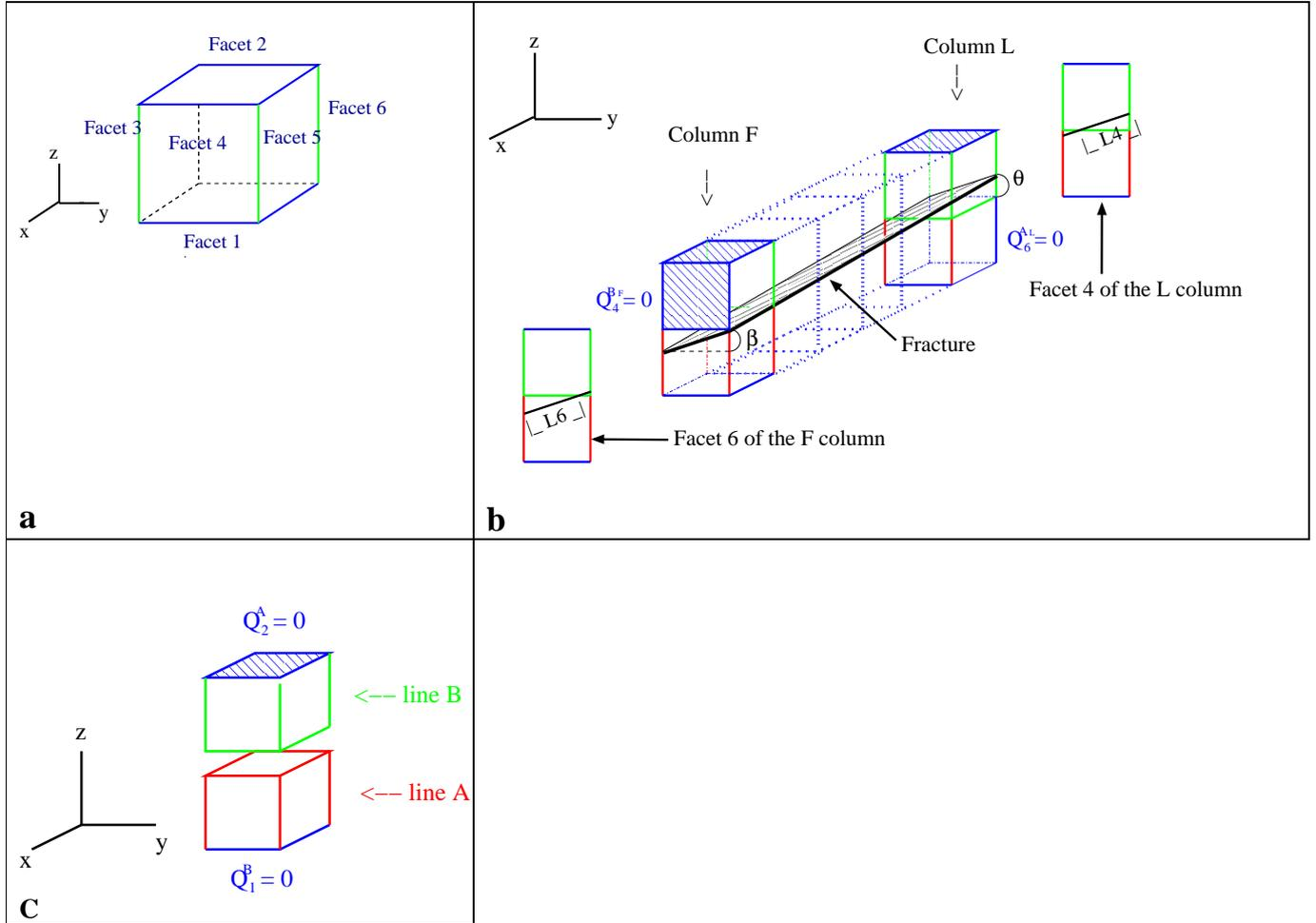
350 Fig. 5. a: facets numbering of a cubic mesh for flux calculations; b: fracture location in a set of
