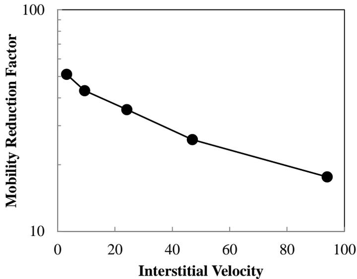
Figure 7: Mobility Reduction Factor evaluated from the performance ratio between foam and gas/water co-injection  $MRF = \Delta P_{\text{foam}} / \Delta P_{\text{water-gas}}$ . The  $\Delta P_{\text{water-gas}}$  is extracted from the linear regression of raw data (Figure 5).
