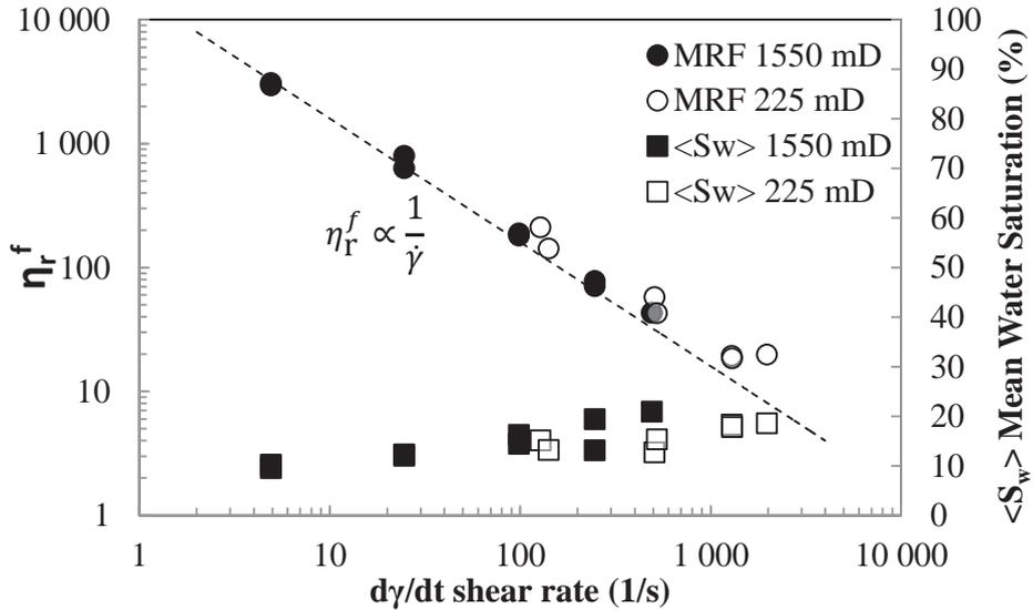
Figure 8: The foam relative viscosity  $\eta_r^f$  (circles) and the mean water saturation  $\langle S_w \rangle$  (squares) vs. the shear rate  $\dot{\gamma}$  computed from eq. (2) in Clashach sandstone at 30°C and a pore pressure of 10 bar. The full symbols represent data for a 1550 mD sandstone with a porosity about 20%. The empty symbols for 225 mD with a porosity about 12%. The dotted line corresponds to the equation  $\eta_r^f = 16000/\dot{\gamma}$ .
