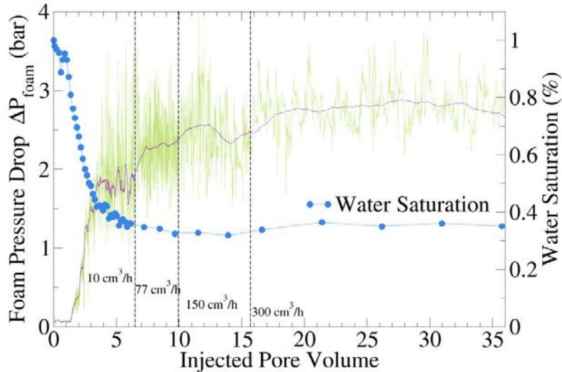
Figure 6: Dense supercritical CO<sub>2</sub>-foam generation in a 820 mD Clashach sandstone. The line in dark purple is a running average of 200 points of the raw pressure drop measurement represented here in light green. The full circles represent the mean water saturation along the core. Data are plotted against the total injected pore volume and thus not linear in time as the total flow rate was increased from 10 to 300 cm<sup>3</sup>/h.
