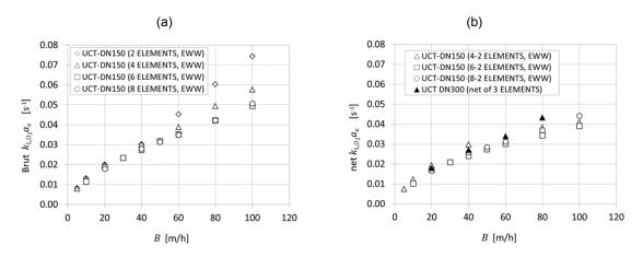
Figure 4.  $k_L a_e$  measured with extra wall wipers (EWW) different bed heights in the UCTP-DN150 columns at  $F_s = 0.02 \sqrt{Pa}$  (a) brut values and (b) net values.
