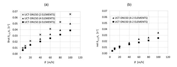
Figure 3.  $k_L a_e$  measured with original wall wipers only for different bed heights in the UCTP-DN150 column at  $F_s = 0.02 \sqrt{Pa}$  for (a) brut values and (b) net values.
