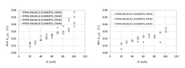
Figure 5.  $k_L a_e$  measured with extra wall wipers (EWW) for different bed heights in the IFPEN-DN146 column at  $F_s$ =0.65  $\sqrt{Pa}$  (a) brut values and (b) net values.
