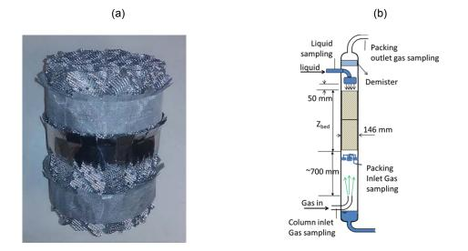
Figure 1: Specifics of the set-up in the IFPEN-DN146 column: (a) packing element with one extra saw-tooth wall-wiper (EWW) and (b) schematic of the column with two packing layers.
