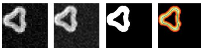
Fig. 1 - Example of processing and analysis of MRI image. From left to right : initial image (resolution 47 \mu\text{m} \times 47 \mu\text{m} ), increase of resolution by numerical interpolation (resolution 14 \mu\text{m} \times 14 \mu\text{m} ), automatic segmentation, distance function calculation (red to yellow colors) and medial axis extraction (blue color)
