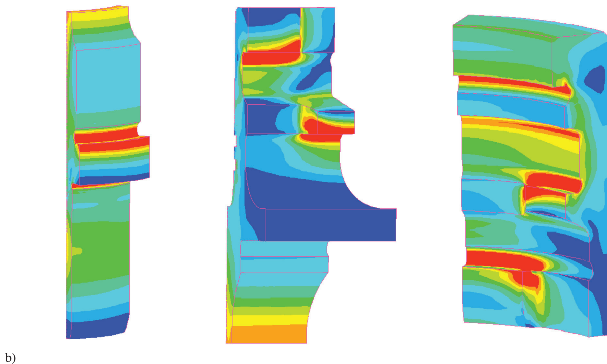
Figure 2b Von Mises stress iso-values in the HP Clip connector. Areas in red exceed the minimum yield strength.
