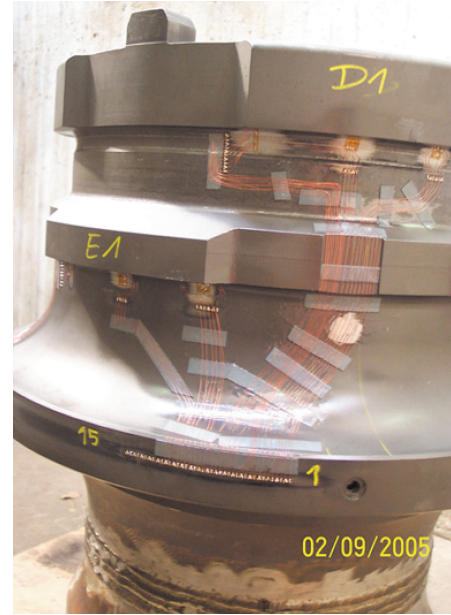
Figure 5 Gage cabling of the female member.
