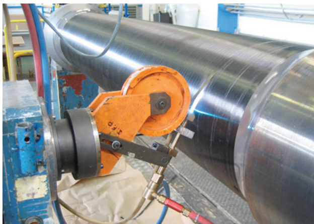
Figure 11 Hybrid pipe during manufacturing process.
