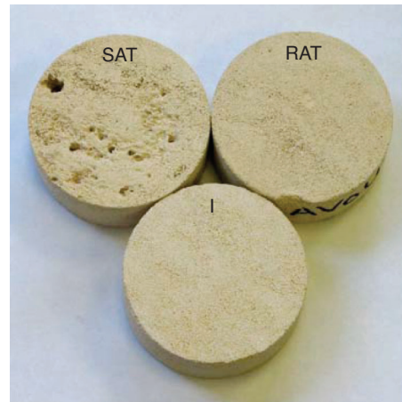
Figure 5 Picture of intact and altered Lavoux limestone samples (I = Intact sample, SAT = sample submitted to a Standard Acid Treatment, RAT = sample submitted to a Retarded Acid Treatment).
