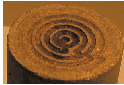
Figure 4 End effects induced by chemical alteration on transition zone samples.
