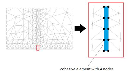
Figure 2. the mesh around the cohesive zone
