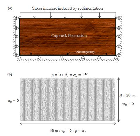
Figure 1. (a) conceptual model and mechanical boundary conditions, (b) finite element method (FEM) numerical simulation model with several vertical predetermined fracture paths,  $\alpha = \frac{b}{\frac{3(1-\nu_r)K_r}{M(1+\nu_r)}+b^2}\sigma_a$
