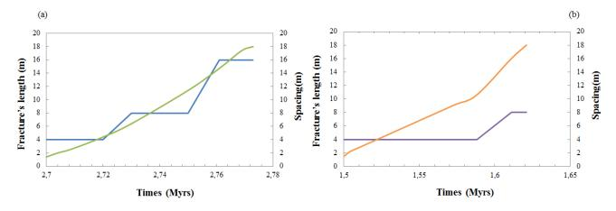
Figure 5. Evolution of fracture's length and of the average spacing between fractures in a ductile caprock (a) and in a brittle caprock(b)
