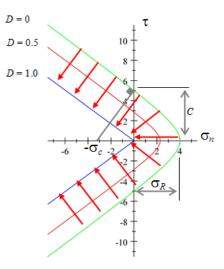
Figure 3. Evolution of the failure criterion from intact cohesive fracture to final damage fracture (*Pouya and Bemani* 2015)
