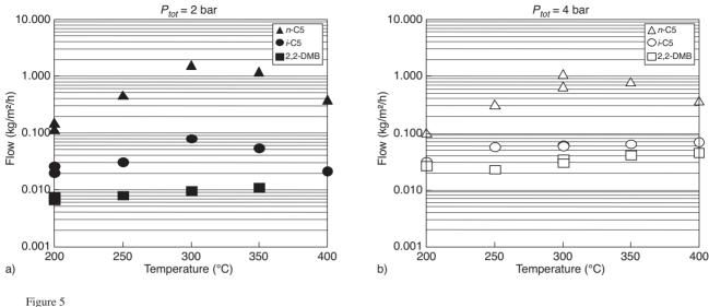
Multi-component permeation tests: fluxes of the various compounds across the membrane as a function of temperature and total pressure.
