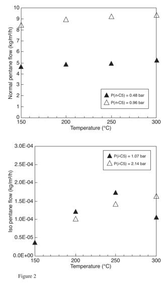
Pure compound permeation tests: graphs of normal pentane (n-C5) and isopentane (i-C5) fluxes *vs* operating conditions.
