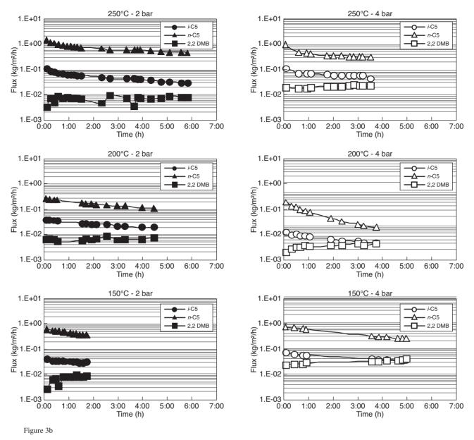
Fluxes of normal pentane (*n*-C5), isopentane (*i*-C5) and 2,2-dimethylbutane (2,2 DMB) against time at various "Total pressure/membrane temperature" pairs.
