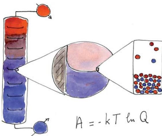
even showing the capillary rise phenomenon) and the macro-scale (illustrated with a distillation column). The well-known Massieu relation  $A = -kT \ln Q$  makes the link between the equations of state (expressed from the Helmholtz energy,  $A$ ), and statistical mechanics (represented by the canonical partition function,  $Q$ ). At the same time, it illustrates the essential relationship between fundamental research (molecular approaches) and applications (process or product design).
