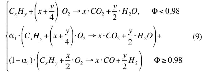
With the conservation of the atom number of C, H and O and the fuel/air equivalence ratio  $\Phi$ , it is possible to define the parameters  $\alpha_1$ , as follow:
