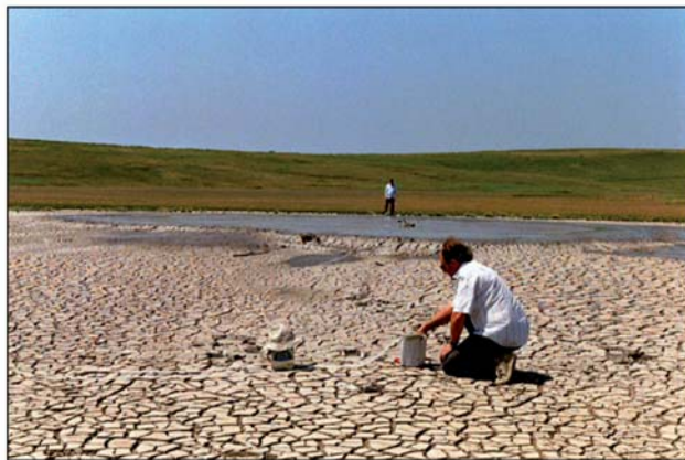
Figure 10 Central Lake: gas sampling with the "Chapka Monomaha" 25 m away from the bubbling point occurring at the centre of the lake.
