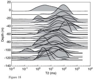
Qualitative pore size distribution of well C1 cores. Time T2 is directly related to the pore size and the signal amplitude is the approximate contribution of a given pore size to the sample porosity: unimodal to bimodal pore size distributions are observed with a very variable spreading from one sample to another.
