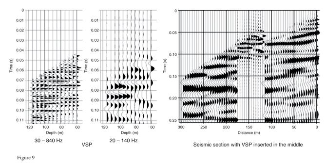
Results of the well seismic survey: calibration of the reflection survey.
