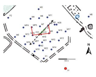
The Experimental Hydrogeological Site - Location of wells: cored wells C1 (reference central well) and C2 are shown in red; the red plain line is a correlation line between wells studied herein; the black dotted line represents the in-line profile of the seismic survey described in the next section of this paper.
