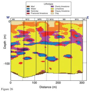
West-East facies cross-section of the Site: a poor connectivity of the conductive facies is expected.
