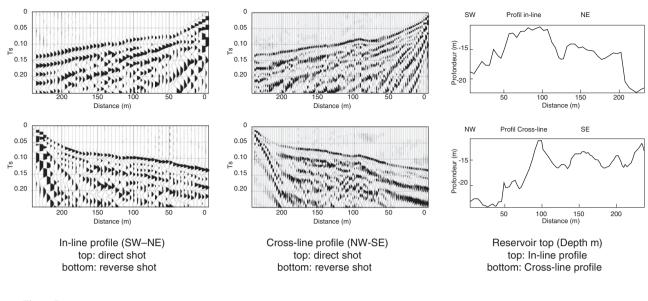
Results of the refraction survey: evidence of an irregular marker above the aquifer.
