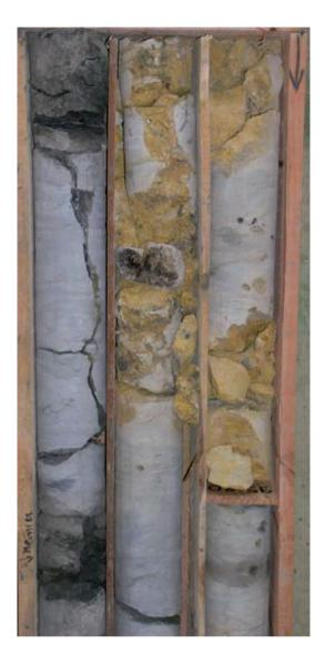
Cores from C2 well at about 97 m depth: clay material is filling the upper "damaged" zone (karst residue?); a vertical fracture is observed between two marly (dark) layers in the lower core.
