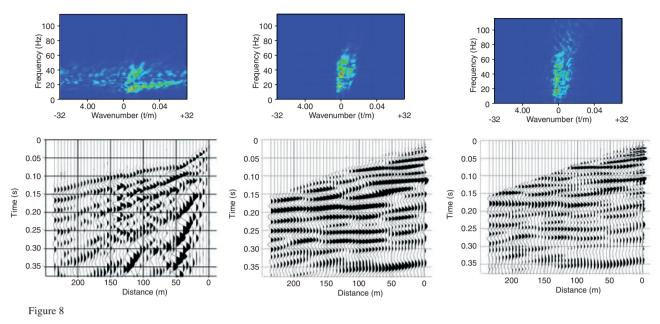
Results of the reflection survey: hardly-detectable reservoir markers as the result of a specific treatment procedure.
