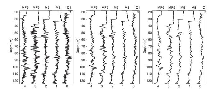
Acoustic velocity profiles of well C1 and neighbouring wells (note that the sharp discontinuity visible in all 5 wells, at a depth varying between 21 m for well C1 and 38 m for well MP5, corresponds to the bottom limit of the steel casing set in the upper section of each borehole).
