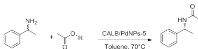
Figure 23. DKR of a racemic amine into enantiopure amide catalysed by a nanobiohybrid. Adapted from Ref. [93].
