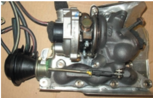
Picture 3 Exhaust manifold.
