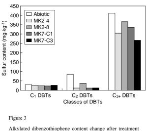
Alkylated dibenzothiophene content change after treatment of a moderately-hydrodesulfurized diesel oil (sample 103).  $C_3$ + DBTs =  $C_3$  and higher alkylated  $C_x$ -DBTs.
