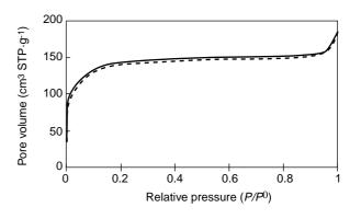
Nitrogen adsorption (—) and desorption (---) isotherms of the mesostrutured alumina synthesized in the presence of sodium dodecyl sulfate and calcined at 450°C.
