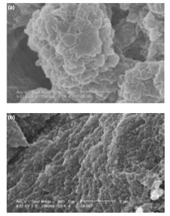
Scanning electron micrographs of samples synthesized by way A; a): at a final pH = 5; b): at a final pH = 10.
