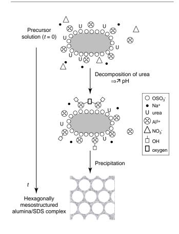
Scheme of the mechanism of formation of the mesostructured alumina synthesized in the presence of sodium dodecyl sulfate.
