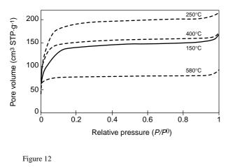
Nitrogen adsorption isotherms of the mesostructured alumina calcined by SCTA at 150, 250, 400 and 580°C.
