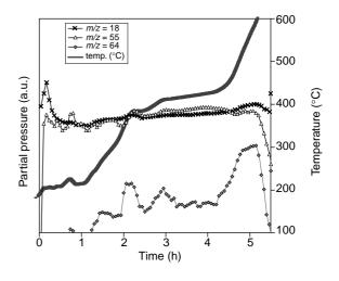
SCTA curve and main mass spectrometry signals of sodium dodecyl sulfate.
