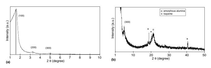
X-ray powder diffraction patterns (CuK<sub> $\alpha 1$ </sub> radiation) of the alumina synthesized by way A at pH = 10; a): for 1° < 2  $\theta$  < 10°; b): for 1° < 2  $\theta$  < 50°.
