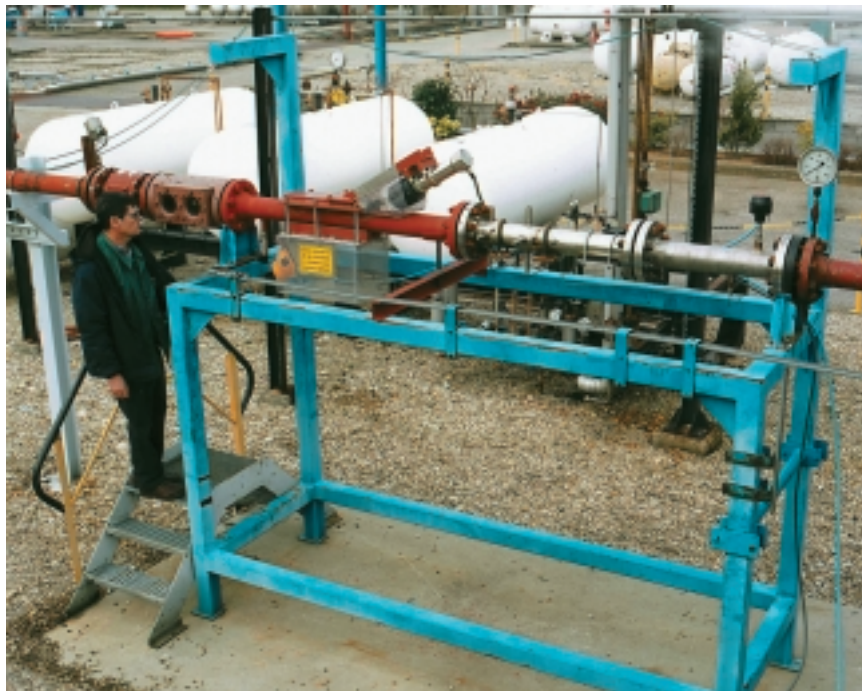
Figure 1b View of the reference venturi meter spool piece with the gamma densitometer and the flow visualisation window.
