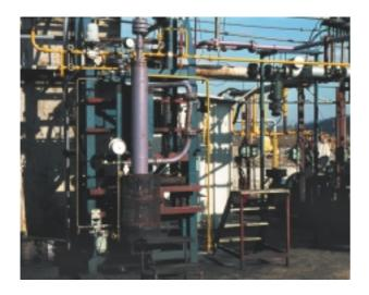
Figure 1 The first helico-axial pump prototype under tests.
