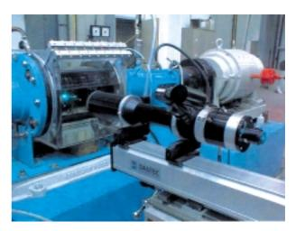
Figure 4 Laser Doppler anemometer.
