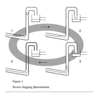
the liquid. Finally, the gas arrives at the top of the riser and the pressure rapidly decreases causing liquid flow down. And so on.
