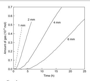
Figure 5 Permeation curves for MDPE at 80°C and 4 MPa of CO<sub>2</sub>.
