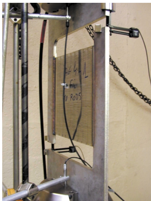
Figure 9 Experimental setting of the shear test.
