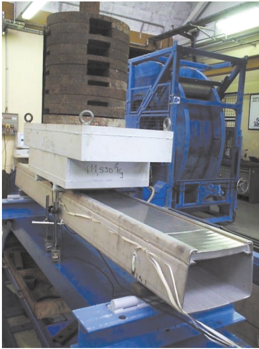
Figure 19 Experimental setting of the four-points bending test on panel.
