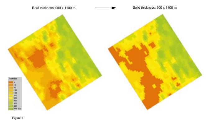
Temis 3D: Backstripping. During the backstripping, the real thickness maps are transformed into solid thickness grids.
