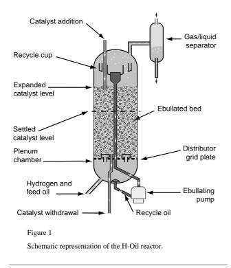
distributor and grid plate. The height of the ebullated catalyst bed is controlled by the rate of liquid recycle flow. This liquid rate is adjusted by varying the speed of the ebullating pump (*i.e.*, a canned centrifugal pump) which controls the flow of ebullating liquid obtained from the internal vapor/ liquid separator inside the reactor.
