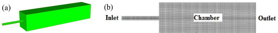
23 24 Fig. 19 Schematic and mesh distribution of a typical injector (a) Schematic; (b) Mesh (204800 cells, 25 the minimum size is 10 \mu\text{m} ).
