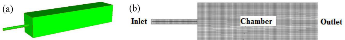
22 23 24 Fig. 19 Schematic and mesh distribution of a typical injector (a) Schematic; (b) Mesh (204800 cells, 25 the minimum size is 10 \mu\text{m} ).
