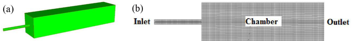
Fig. 19 Schematic and mesh distribution of a typical injector (a) Schematic; (b) Mesh (204800 cells, the minimum size is 10 \mu\text{m} ).
