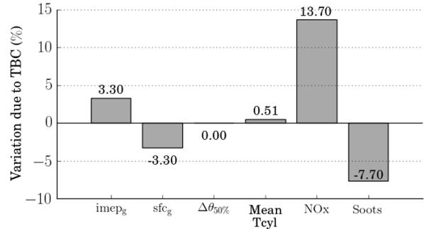
**Figure 15.** Variations in % of gross  $imep$  and  $sfc$ ,  $\Delta\Theta_{50\%}$ , mean cylinder gas temperature and mass of NOx and soots at the start of exhaust for the case with TBC compared to the baseline.
