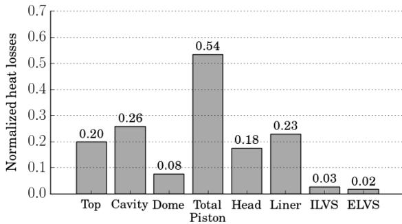
Figure 7. Normalized heat losses through the cylinder walls. ILVS: intake lower valve surface; ELVS: exhaust lower valve surface.
