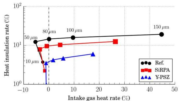
Figure 11. Heat insulation rate against intake gas heat rate for 5 values of insulation thickness and 3 coatings. "Ref." represents the reference coating considered in this study.
