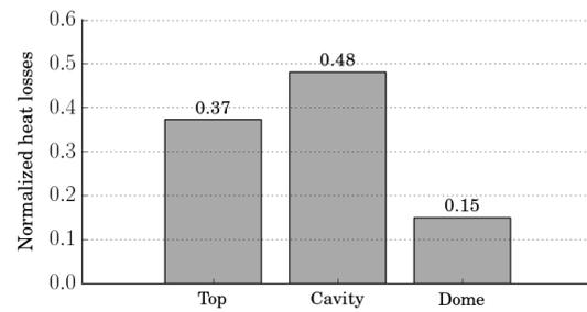
Figure 6. Heat losses rate (left) and normalized heat losses (right) through piston surface.
