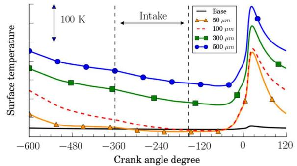
Figure 10. Surface temperature profiles for various thicknesses of the reference coating.
