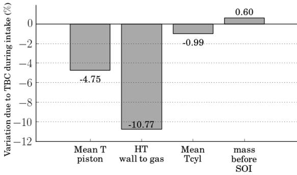
**Figure 13.** Relative variation due to TBC of mean piston temperature, integrated heat transfer from wall to gas during intake, mean in-cylinder gas temperature during intake and in-cylinder mass (before SOI, start of injection), compared to the baseline.
