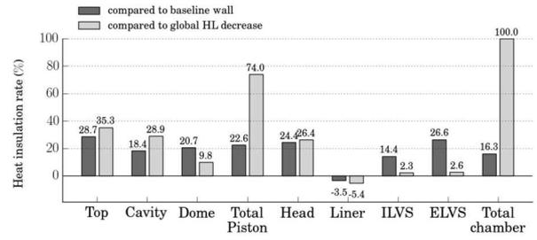
**Figure 14.** Heat insulation rate due to coating compared to baseline wall (dark grey) and compared to global heat losses decrease (light grey). ILVS: intake lower valve surface; ELVS: exhaust lower valve surface.
