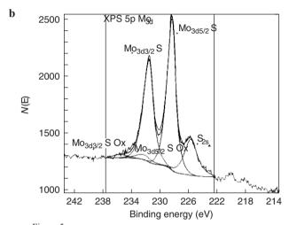
Figure 5 XPS spectra of MoS<sub>2</sub>/Al<sub>2</sub>O<sub>3</sub> catalysts, partially or totally sulphured.
